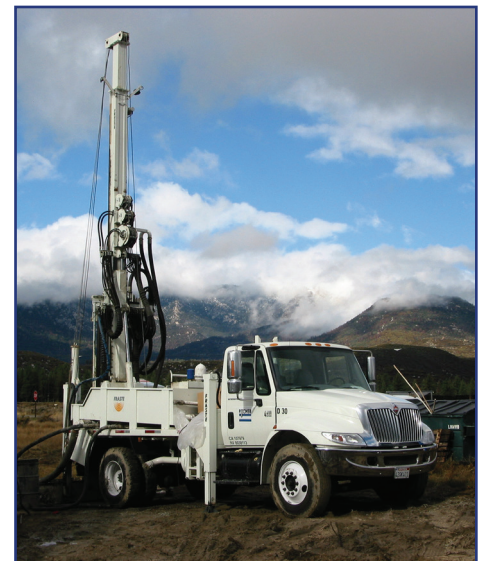
The Fraste MD/XU is a top head drive rotary rig with make up/break up clamps also capable of rock coring.
